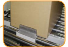
Standard indexing gate assures only one case at a time enters the machine
