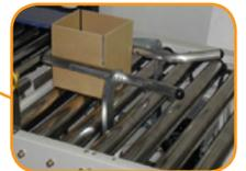
Optional powered centering & indexing conveyor lets the machine control case flow
